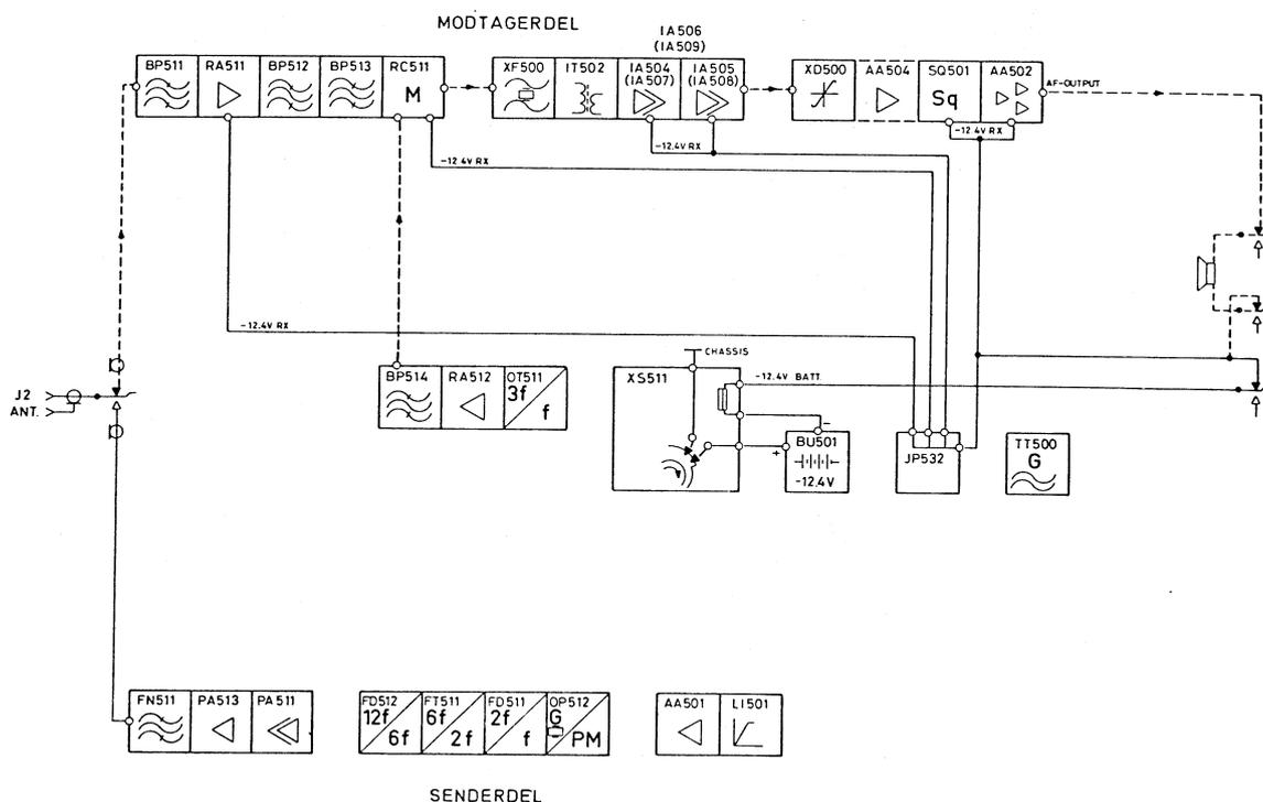
voltage and ADC-controlled voltage from junction panel JP531. Besides, the antenna is connected to the transmitter RF output and the speaker-microphone to the AF input.
