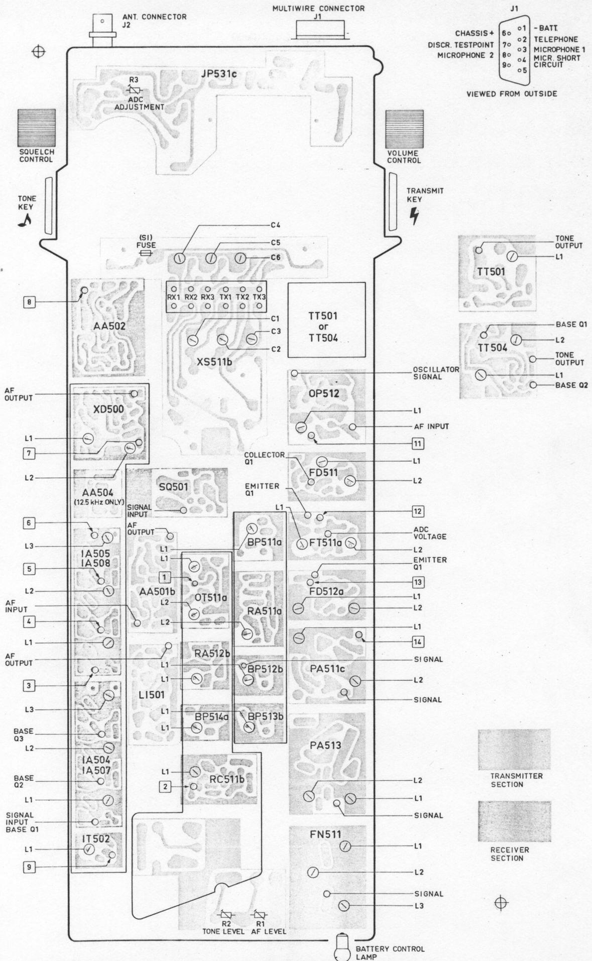
LOCATION OF TEST POINTS AND ADJUSTABLE COMPONENTS IN CQP510
