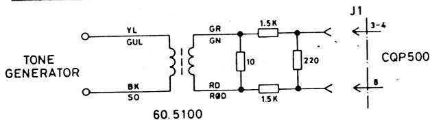
Connect tone generator via matching transformer to pins 3/4 and 8 of connector J1.
